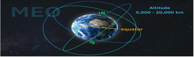
• To increase coverage, sometimes constellations like this, consisting of several of the same or similar satellites, are launched together to create a 'net' around Earth.
